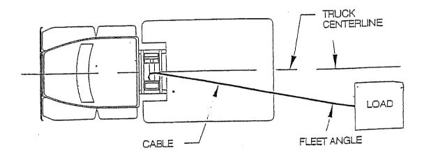
The fleet angle should be kept as small as possible to insure proper spooling and to maximize cable and winch life. To promote even cable spooling, keep the fleet angle below three degrees. Whenever possible, spool through a block at the back of the truck body. Never pull directly against the flange of the winch cable drum as this may cause the cable or the winch to be structurally compromised.
